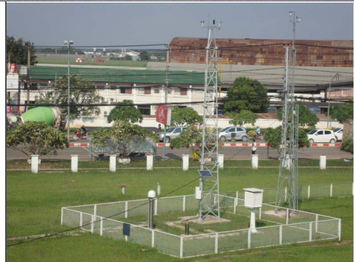
Typical automated surfaces observation station with Conventional instruments
